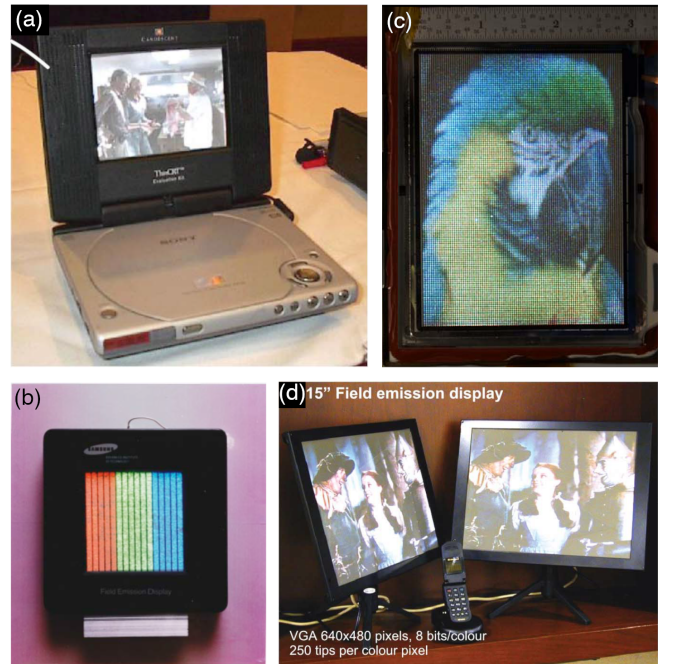
Fig. 5.2: Field emission display prototypes. (a) Sony portable DVD player, adapted from [31]. (b) Samsung 4.5" FED, adapted from [44]. (c) Motorola 4.6" FED, adapted from [46]. (d) Motorola 15" 640 × 480 FEDs and handsets, adapted from [31].
